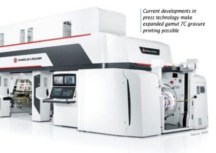
it holds register during the production run. The register control system must guarantee that the gravure formes print the separated colours precisely in position on top of or alongside each other without any register differences. If this is not the case it becomes apparent in
