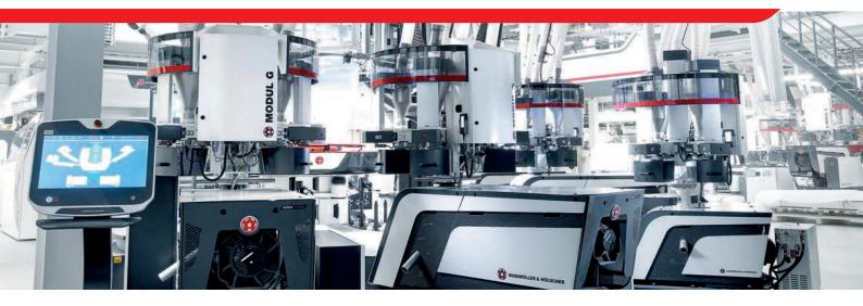
The new automation modules TURBOSTOP and TURBOSTART support the operator in shutting down and starting up the line in a simple seven-step approach. The intelligent interaction between software and dedicated hardware components ensure an automatic process from shutting down all machine components, securing the film in the line and starting up all components again, until the line is running again.
