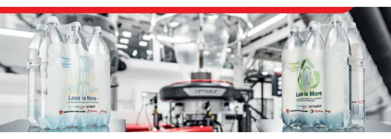
The new collation shrink film presented by W&H is using recycled PE taken from post-consumer waste. The packaging keeps its optical and mechanical properties.
