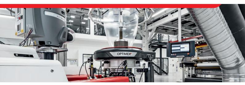
The OPTIMEX" is suited for a wide range of films with 3- or 5-layers and combines high output rates with outstanding film quality. Many components originate from the VAREX" high-end product family and have been adapted for **OPTIMI**zed **EX**trusion, especially for PE products.
