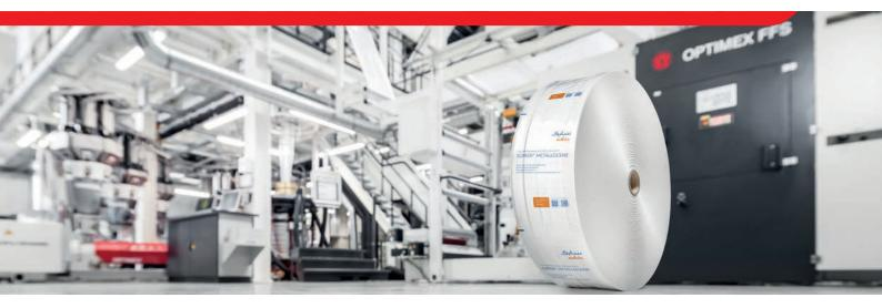
This Heavy Duty Sack (HDS) film is produced at a groundbreaking production output with excellent film tolerances and roll quality. The film meets the requirements of all downstream processes from inline printing, side gusseting and embossing to filling and stacking of the finished bags.
