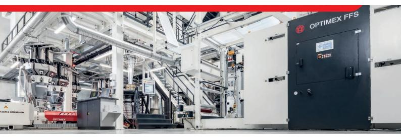
The OPTIMEX" FFS has been optimized to overcome the three main factors limiting the line output of the most commonly used recipes in Heavy Duty Sack (HDS) film production. The improved bubble stability with a new high performance cooling package leads to 15–20 % output increase.
