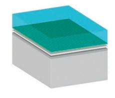
20 µm BOPP film (counter printed) Adhesive
