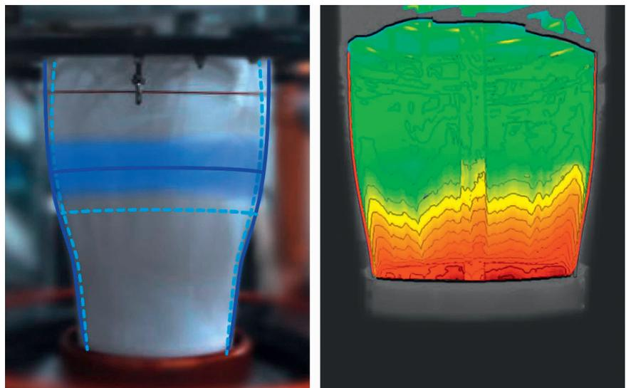
**Fig. 3.** Inline recording of the cooling behavior in the film bubble. The setpoints for the bubble shape and the frost line height are represented by broken lines, and the current values by continuous lines. © W&H
