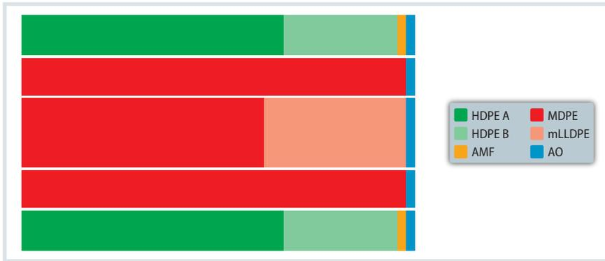
**Fig. 1.** Film structure of a MDO-PE 5-layer film. The height of the bar represents the thickness of the layers, the color of the bar represents the different raw materials, and the width of the bar represents the proportion of the raw material in the respective layer. Source: W&H; graphic: © Hanser
