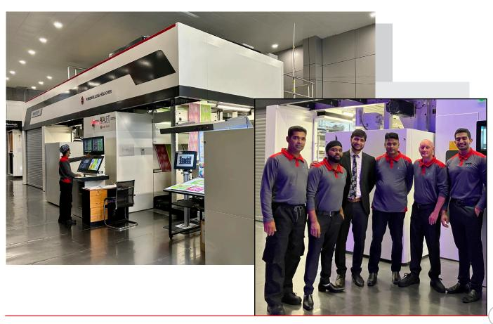
During the Covid period in 2021, ALFT packaging installed the CI Flexo press MIRAFLEX II. The local staff from the W&H Indian office completed the installation, commissioning, and startup. Within a short period, the press was operating at 500 m/min, its maximum speed. The press has a ton of specific features that cut down on startup and changeover waste and changeover time. It is the most sophisticated and feature-rich printing press delivered to the nation.
