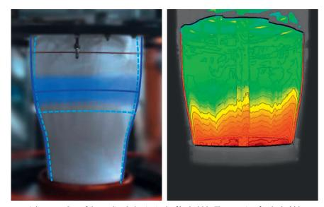
**Fig. 3.** Inline recording of the cooling behavior in the film bubble. The setpoints for the bubble shape and the frost line height are represented by broken lines, and the current values by continuous lines. © W&H
