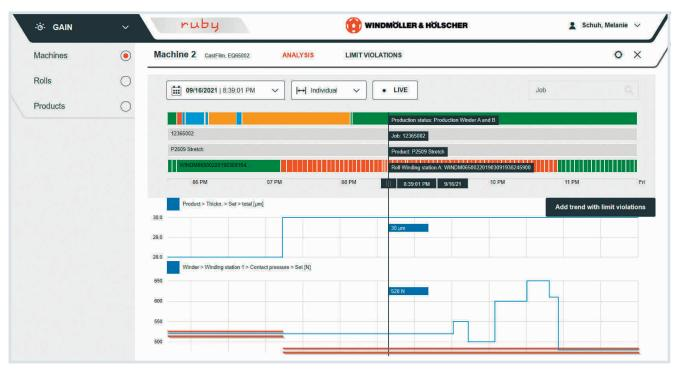
Fig. 2. The limit violation shows that the contact pressure still needs to be adjusted. © W&H
