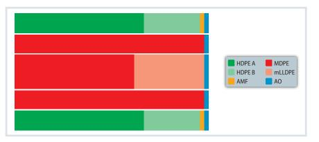
**Fig. 1.** Film structure of a MDO-PE 5-layer film. The height of the bar represents the thickness of the layers, the color of the bar represents the different raw materials, and the width of the bar represents the proportion of the raw material in the respective layer. Source: W&H; graphic: © Hanser
